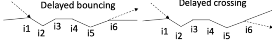
Fig. 6. Overlapping edges ( i_1, i_2, \dots, i_6 ) from P and Q are shown as an intersection chain . i) Delayed bouncing intersection chain: leftmost dotted line is labeled Left|On . The rightmost dotted line is labeled On|Left . ii) Delayed crossing intersection chain: leftmost dotted line is labeled Left|On . The rightmost dotted line is labeled On|Right . The vertices i_1 to i_6 are labeled On|On .
