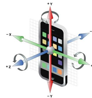
Figure: Gyroscope Axes
