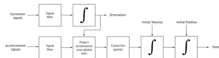
Figure: Strapdown inertial navigation positioning algorithm. Adapted from Woodman.
